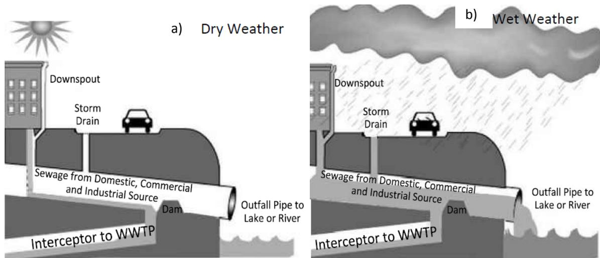
**Figure 1.** a) During dry weather, sewage and commercial wastes do not cause overflows. The waste flows into an interceptor pipe to the waste water treatment plant. b) During wet weather, sewage, commercial wastes and stormwater mix and overwhelm the system. Due to the surge in volume, not all waste gets to the interceptor and therefore it is released to the nearest water body.
